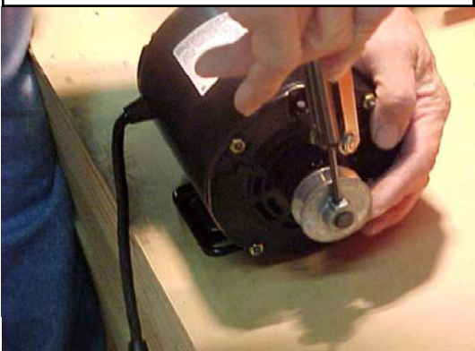
Electric Motor Assembly: Slide pulley onto motor shaft and tighten with Allen Wrench.
