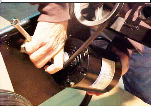
After installing belt onto 2" pulley on motor and 6" pulley on frame, tighten belt by sliding motor assembly down away from 6" pulley. Tighten hex screws with 1/2" wrench.
