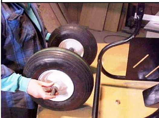
Put wheels on each axle rod end with hub out and stem inside
